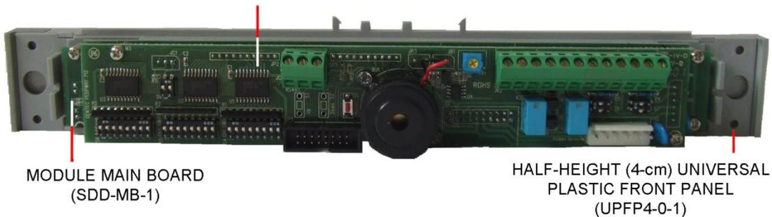
Figure 3.2 Internal View of an Assembled g-Smart Data Display Enhanced™ Module.
