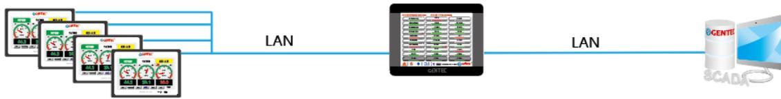
The central alarm, on-site alarms, and the SCADA are communicated with each other through the network connection. The connected network must be in the same local area network.
